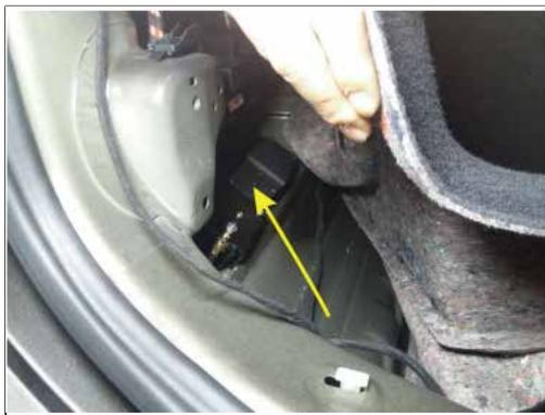
13. The electric suction lock is installed on the right side of the tailgate and fixed with our 3M glue (as shown in the figure)
