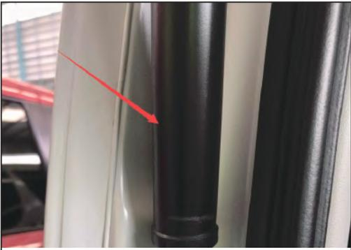
1. Remove the left and right braces of the original car
