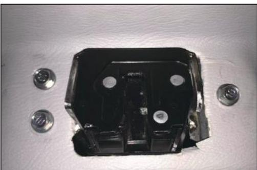
10. Remove the original locks and install our electric suction locks. Fixed with screw
