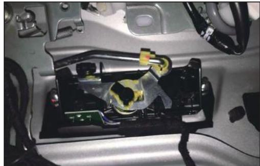
9. Remove the mechanical lock of the original car and install the tail door specially designed by our company Switch key, fixed with original screw
