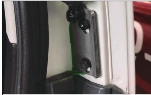
3. Remove the right lower bracket of the original car and install our special bracket
