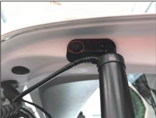
4. Remove the left upper ball head of the original car and install it. Our company specializes in it. The bracket is fixed with our screw
