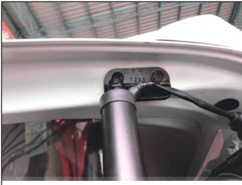
5. Remove the right upper ball head of the original car and install it. Our company specializes in it. The bracket is fixed with our screw
