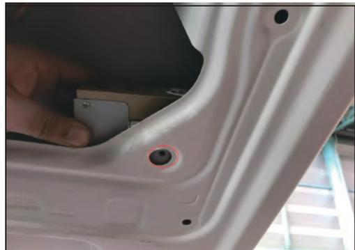
12. The control box is mounted at the rear of the car with screws. Gasket fixation
