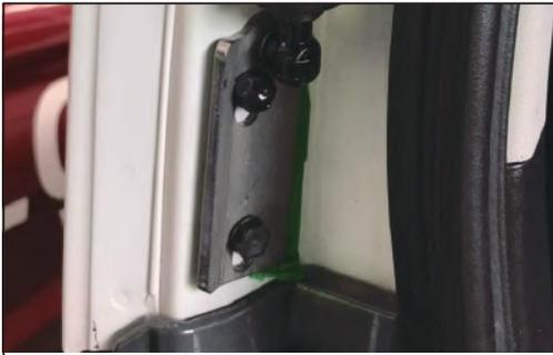
2. Remove the left lower bracket of the original car and install our special bracket
