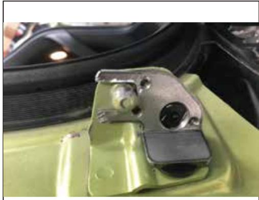
3. Insert our left and right brackets on the original car bracket
