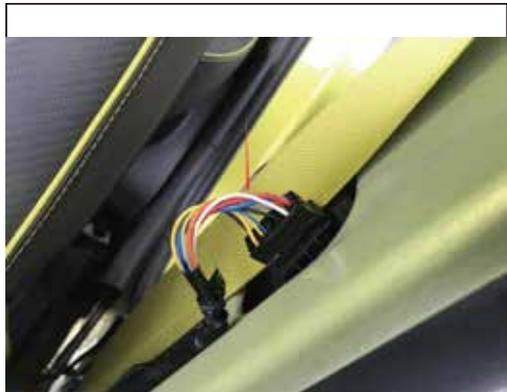
9. Connect the central control wire at the B-pillar of the original car
