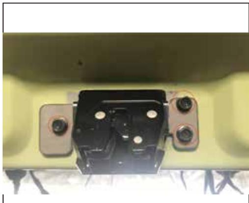
12. Remove the original lock and install our suction lock. Then, fixed with screw.
