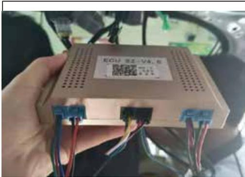
16. Hall wire, central control wire, power wire according to color insert one by one to control box
