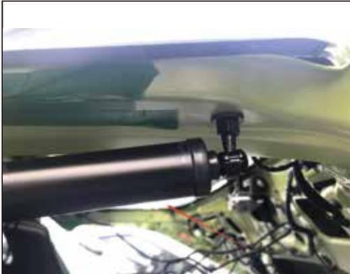
5. Install our left electric pole with the original car ball mount
