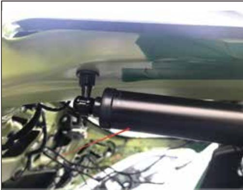
2. Remove the original car right support strut
