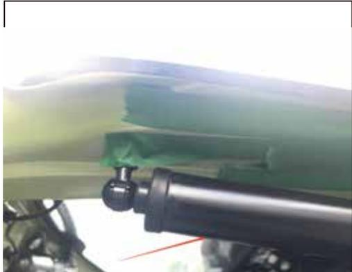
6. Install our right electric pole with the original car ball mount
