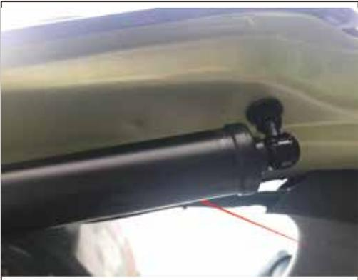
1. Remove the original car left support strut
