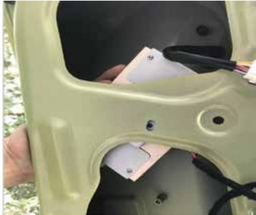
17. Install the control box at the original car tailgate. Fixed with our screw.
