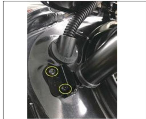
3. Remove the left lower bracket and electric pole of the original car, install the left lower bracket and electric pole of our company
