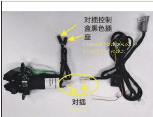
16. As shown in the figure, plug in our electric suction lock socket
