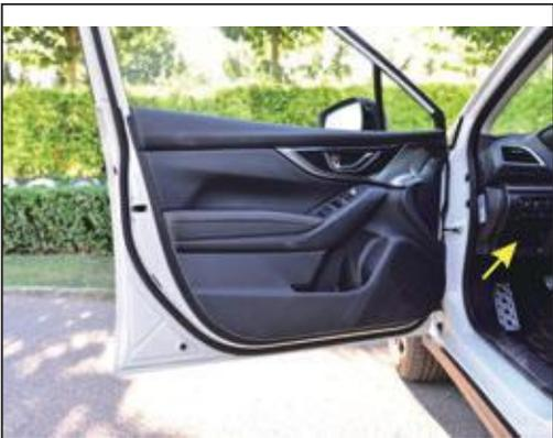
7. Remove the trim board from the main driver compartment and find the power supply
