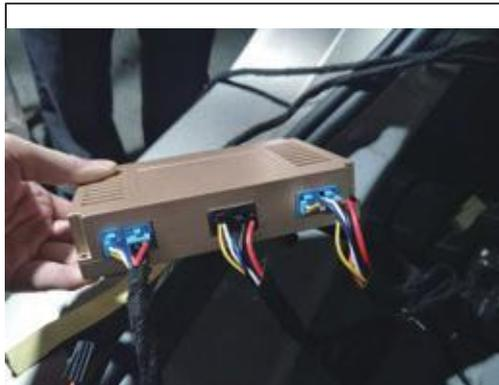
17. Take the Hall cable, power cord and electric suction cable sockets, plug in according to their colors one by one to the control box
