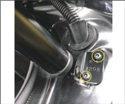
4. Remove the right lower bracket and electric pole of the original car, install the right lower bracket and electric pole of our company
