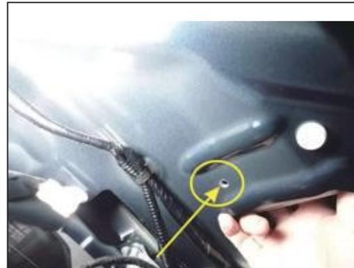
18. Installation position of control box, fixed with company's screw, ring and spring
