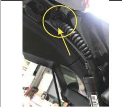
5. After the installation of the electric pole is completed, punch a hole above the ball head, and the electric pole cable goes to the tailgate cover board (the same steps are left and right).
