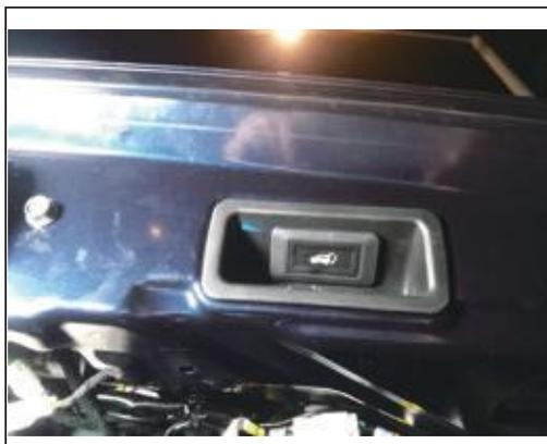
19. Remove the original car trim panel, punch hole and install our company's tailgate switch
