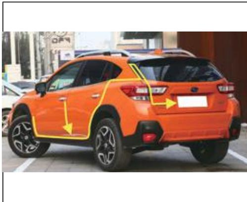
14. The power supply cable and the central control cable run along the car body to the tailgate control box.
