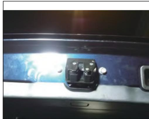
15. Remove the trim board from the trunk and find the original car latch
