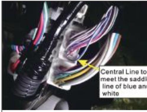
5. The main driving A central column below remove the plaque found, our company yellow Central Line meet the seat blue and white line (the second from bottom in the first row from left to right several holes)
