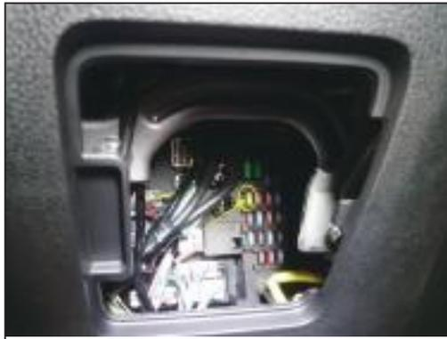
4. Remove the plaque found below main driving power supply, unplug the original car yellow 20 a fuse, plug in our power plug
