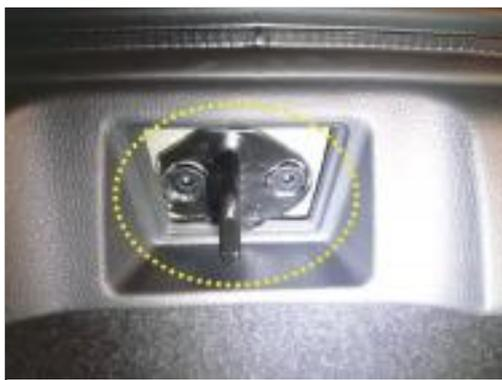
10. Remove the original lock buckle, installing special lock, with screws
