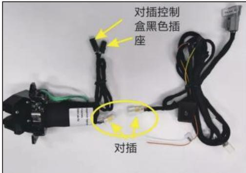
16. As shown in the figure, the socket of the three-way harness is connected to our electric suction socket.
