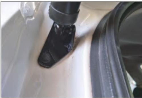
2. Remove the lower left bracket of the original car, replace with our lower left bracket (ball head facing outward), and fix it with the original car screw.
