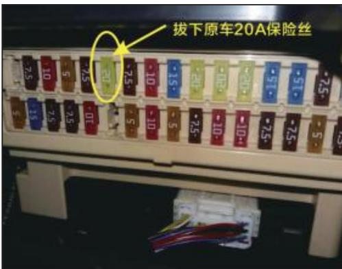
8. Remove the trim board under the driver compartment, pull out the 20A fuse of the original car, and insert our power plug.
