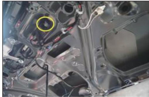
18. Unplug this socket at the tailgate and connect to our front switch socket
