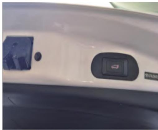
21. Install the tailgate switch at the position shown in the figure
