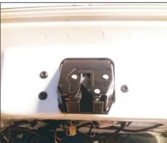
25. Remove the original car door lock, install our electric suction, use the original car screws
