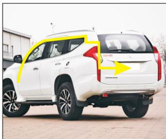
21. The co-pilot's power cable is routed along the yellow arrow line to the tailgate cover
