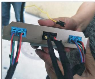
28. control box plug by color plug, pay attention to check whether inserted in place
