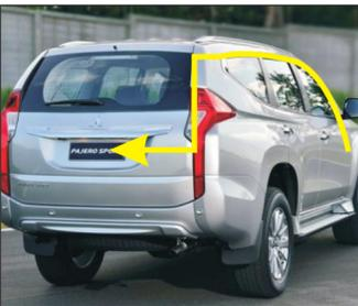
22. Before the main driving switch, the OBD line is routed along the yellow arrow line to the tailgate cover
