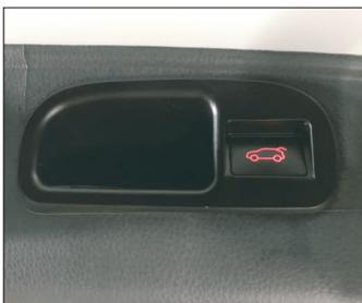
32. Remove the trim plate and install the end button of our company. The rear door socket and the socket of the three-way wiring harness
