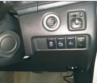
Press the front switch button to open/close the tailgate
