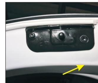
10. Install the left upper bracket of our company, same as the right bracket installation method
