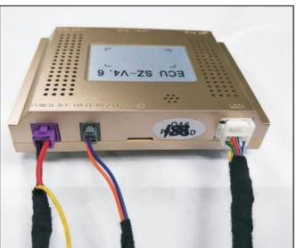
29. White plug of control box inserted, and finally plugged in purple socket
