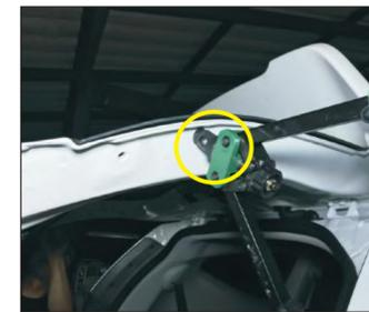
6. In the hole position of the hole, use the rivet gun to rivet
