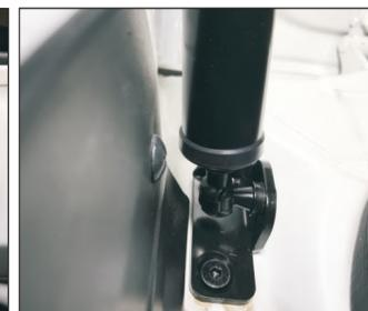
11. Install our company's left lower bracket, (ball head toward the outside of the body) with our
