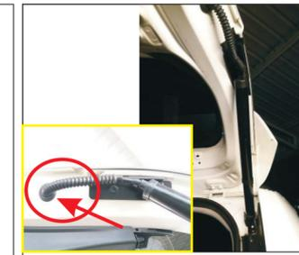
12. In the bracket above the punch strut line through the hole to the tail door cover
