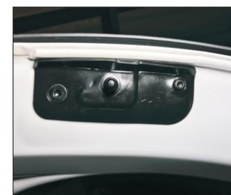
8. Install the right upper bracket of our company. Use the flat head screws of the original hole and the round head screws of our company.
