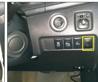
18. Remove the original car empty button, install the front switch button
