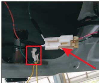
26. Unplug the original car seat at the door lock and insert the three-way adapter socket of our company. The white socket of the electric lock and the socket of the three-way wiring harness are inserted.
