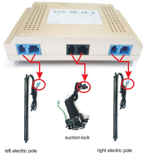
left electric pole suction lock right electric pole
