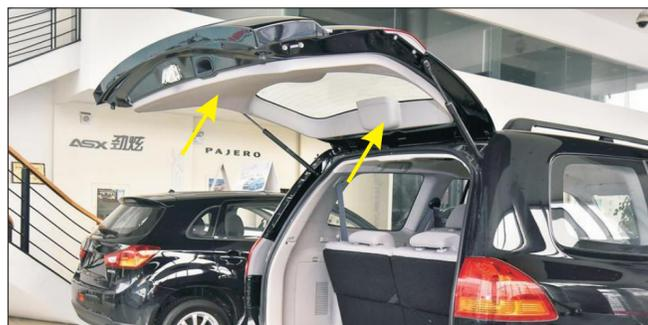
1. as shown in the picture, remove the plaque and the original car electric pole.
