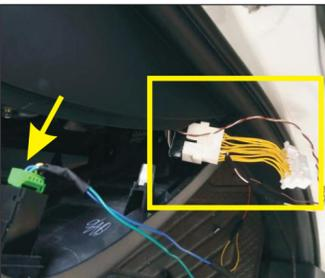
19. As shown in the figure before the switch button plug, find the original car protocol below the switch to plug our OBD
