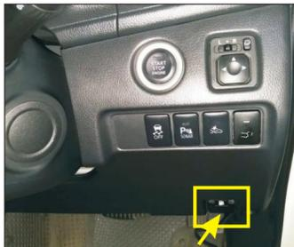
20. OBD insertion below switch before main driving
