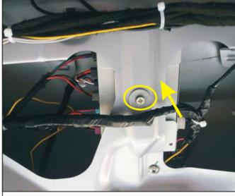
31. Control box installation position, with our screws, gaskets, mesons
