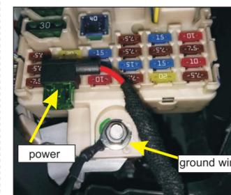
16. Plug in our power socket, the grounding screw below the power supply to our ground wire
