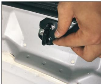
24. Install our special lock, fixed with the original car screws
