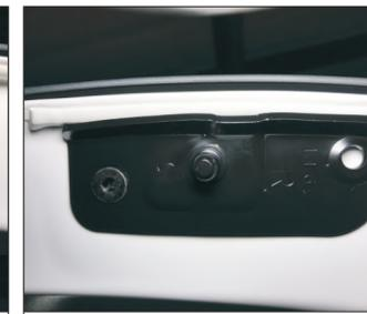
3. Install the special upper right bracket of our company. As shown in the picture, the original vehicle ball head uses our balance screw fixing bracket.
