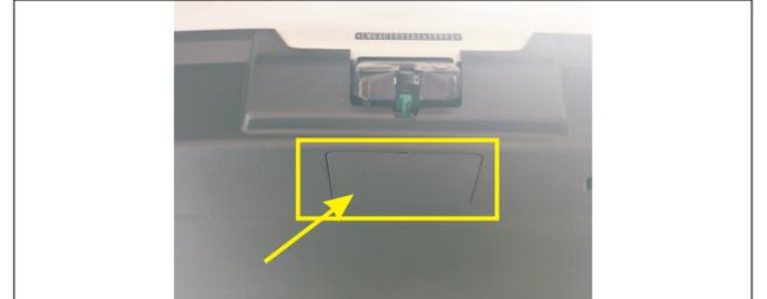
**!** When the tailgate cannot be opened normally, find the original car emergency safety lock in the trunk and open the emergency cover. Pull emergency switch to open
