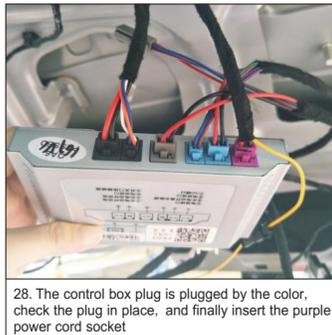
28. The control box plug is plugged by the color, check the plug in place, and finally insert the purple power cord socket
