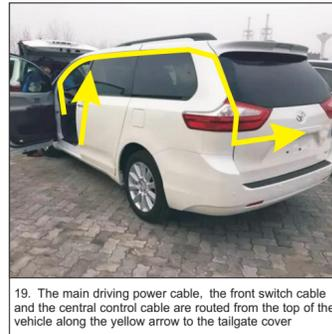
19. The main driving power cable, the front switch cable and the central control cable are routed from the top of the vehicle along the yellow arrow to the tailgate cover
