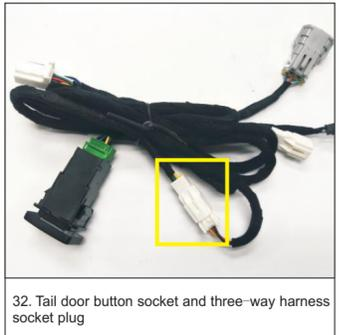
32. Tail door button socket and three-way harness socket plug
