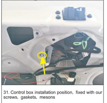
31. Control box installation position, fixed with our screws, gaskets, mesons
