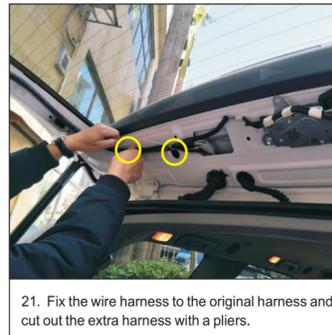
21. Fix the wire harness to the original harness and cut out the extra harness with a pliers.
