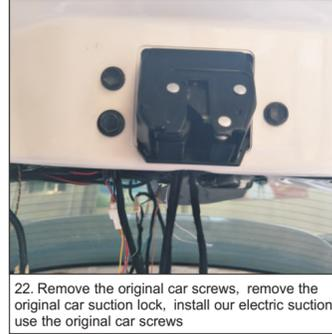
22. Remove the original car screws, remove the original car suction lock, install our electric suction, use the original car screws
