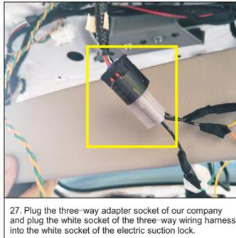
27. Plug the three-way adapter socket of our company and plug the white socket of the three-way wiring harness into the white socket of the electric suction lock.
