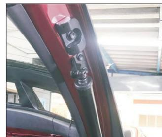
2. Install the company's struts with the right upper bracket of the original car (same as the left and right steps)
