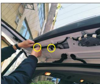
24. Fix the wire harness to the original harness, and cut out the extra harness with a pliers.
