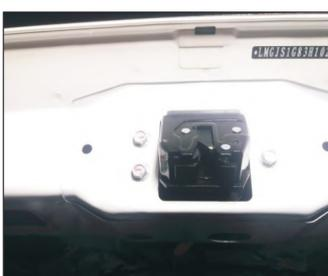
25. Remove the original car screws, remove the original car suction lock, install our electric suction, use the original car screws
