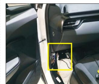
15. Find the original car power and ground under the co-pilot
