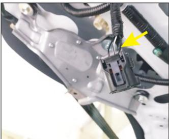
27. Find the original car socket at the tailgate, the two cables thrown by the front switch, and the black cable connecting the terminal housing.
