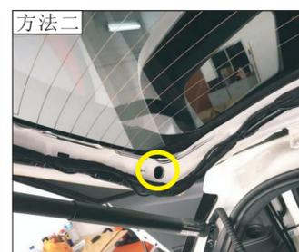
8. Remove the original vehicle rubber plug and punch holes in the yellow circle of the original car, which is conducive to the strut wire alignment (the same as the left and right steps)
