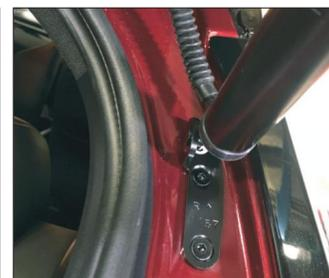
3. Remove the right lower bracket and strut from the original car, install the lower right bracket of our company, engrave with "R", and the arrow faces upwards. The ball head is toward the outside of the body and is fixed with our screws.
