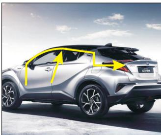
22. The main driving power cable and the central control cable are routed from the top of the vehicle along the yellow arrow to the tailgate cover
