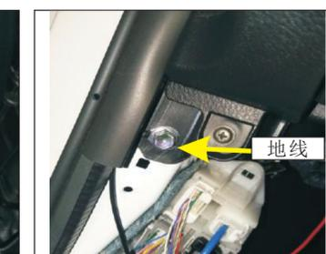
18. Remove the plaque from the lower left side of the co-pilot to find the grounding screw and connect the ground wire.
