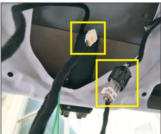
29. Unplug the original car seat at the door lock and insert the three-way adapter socket of our company, and plug the socket of the three-way harness into the electric suction lock socket.
