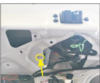
33. Control box installation position, with our screws, gaskets, mesons
