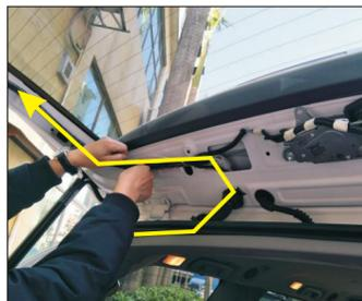
23. The power wire, the front switch wire, and the center wire are routed from the top of the vehicle along the yellow arrow to the tailgate cover
