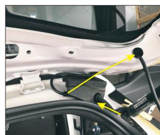
9. The right strut line passes through the rubber stopper of the original vehicle, and goes along the yellow cable to the tailgate cover (same as the left and right steps)
