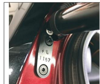
4. Remove the left lower bracket of the original car, install the left lower bracket of our company, engraved with "L", the arrow is upward, the ball head is toward the outside of the car, and it is fixed with our screws.
