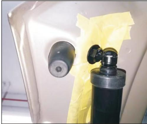
2. Remove the original car upper ball head, the installation I left superior ball head, the ball head with a gasket we deserve
