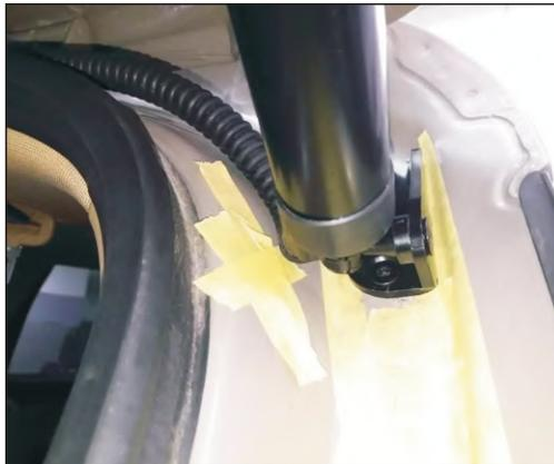
5. Remove the original car right bracket, we lower bracket, installation poles (the line ends of the poles down)
