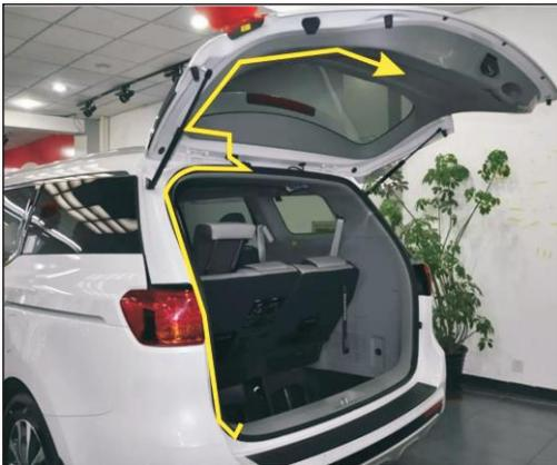
16. Electric door suction line go line to end cover plate
