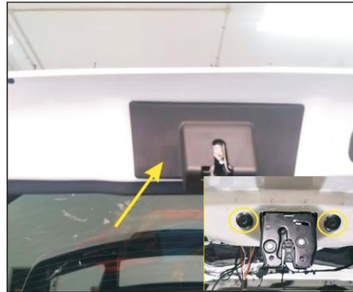
15. Abort the original screw, remove the original car lock, installed on our electric absorption, use the original car screws
