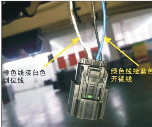
14. At the tail door locks unplug the saddle to take the orange line in the seat of the white line, green line after the blue line
