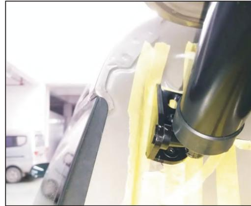
3. Remove the original car bottom bracket, we lower left bracket, installation poles (the line ends of the poles down)
