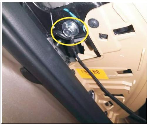
10. In the main drive side remove the plaque, find the ground
