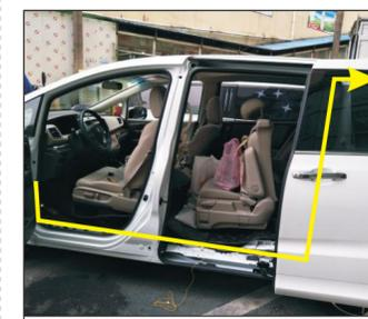
17. The main driving power cord and switch line from the body before walking down the yellow arrow below line to end door cover plate
