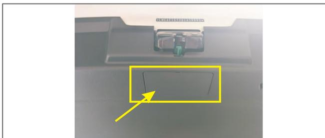
! When the tailgate cannot be opened normally, find the original car emergency safety lock in the trunk and open the emergency cover. Pull emergency switch to open
