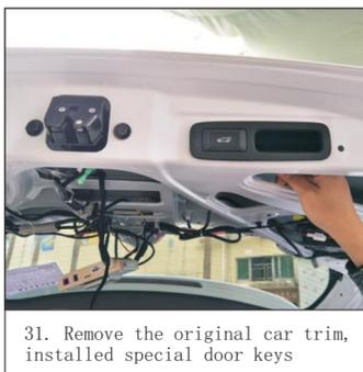
31. Remove the original car trim, installed special door keys
