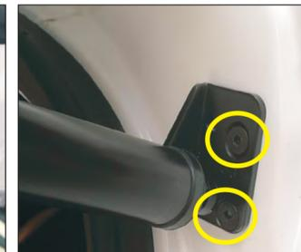
5. Remove the original car bottom bracket, installation we lower left bracket (ball head toward the outside), with our screws
