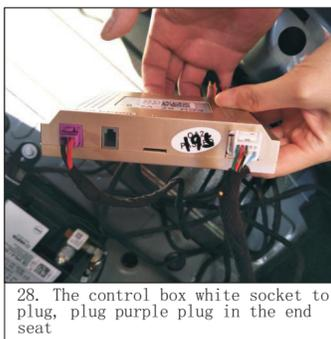
28. The control box white socket to plug, plug purple plug in the end seat
