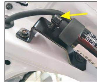
2. Remove the original car right bracket, installation of upper bracket, In the original car screws
