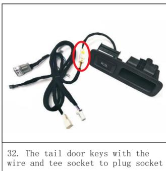
32. The tail door keys with the wire and tee socket to plug socket
