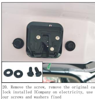
20. Remove the screw, remove the original car lock installed ICompany on electricity, use our screws and washers fixed
