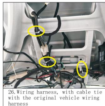
26. Wiring harness, with cable tie with the original vehicle wiring harness
