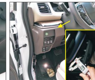
13. Remove the plaque to find the original car white socket
