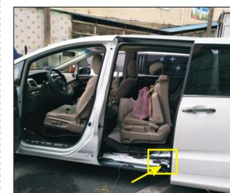
15. The back wheel on the left side of the lid of the waste footplate, find the original car central control
