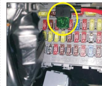
10. Remove the original car fuse, plug in our power plug
