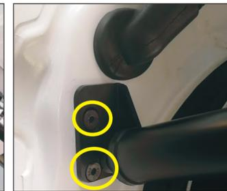
3. Remove the original car right bracket, installation we lower bracket (ball head toward the outside), with our screws
