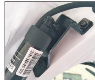
4. Remove the original car left bracket, installation of upper bracket, In the original car screws
