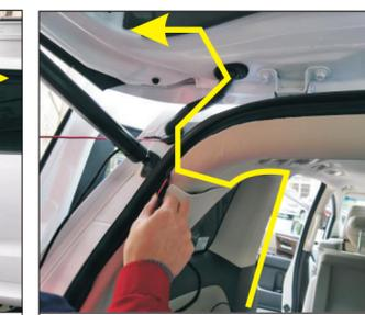
18. The main drive and control the power cord, switch before walked along the yellow arrow line to end door cover plate
