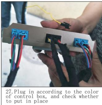
27. Plug in according to the color of control box, and check whether to put in place
