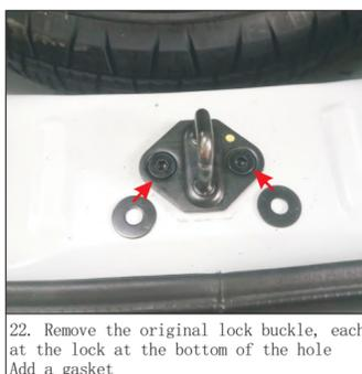
22. Remove the original lock buckle, each at the lock at the bottom of the hole. Add a gasket
