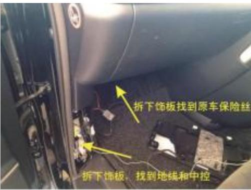
7. Find the power, ground and central control lines as shown in the co-driver compartment
