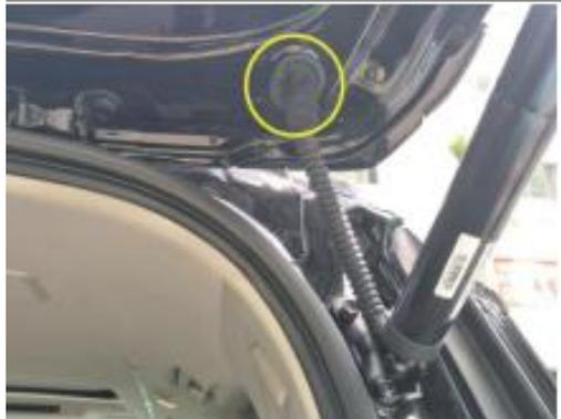
6. Remove the rubber plug of the original car and punch it with our drill bit. Our Hall wire passes through the rubber plug hole and goes to the tailgate cover.
