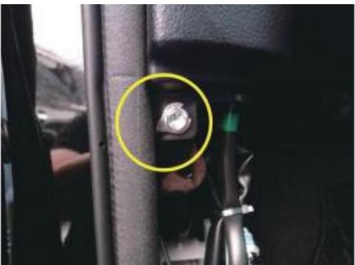
9. Locate the ground screw under the driver compartment and connect the ground wire.
