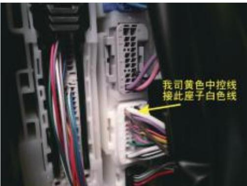
10. Find the central control under the ground wire. Our yellow color control wire is connected to the socket's white color wire.
