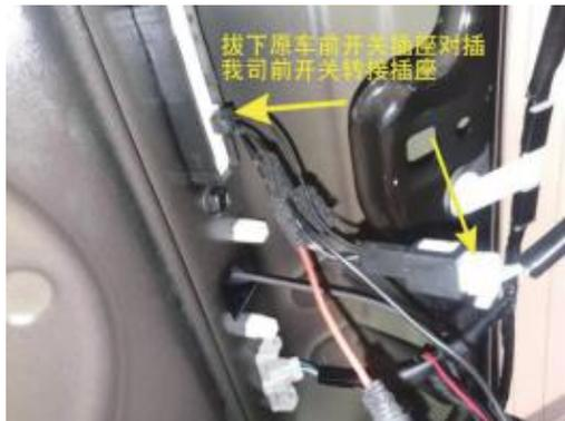
12. On the back of the original car tailgate opening button, find this socket and plug in our front switch adapter socket
