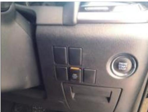
11. Remove the dummy button at the driver compartment according to the owner's habit, and install our front switch button.
