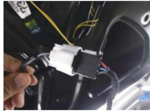
15. Unplug the original car socket at the door lock and insert it into our three-way adapter socket.
