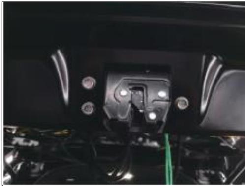
14. Remove the original door lock, install our electric suction lock, fix it with the original car screws
