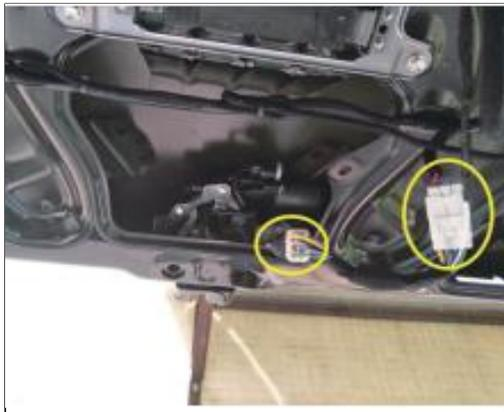
13. Locate the socket at the original door lock, unplug the original car socket and plug it into our three-way adapter socket.
